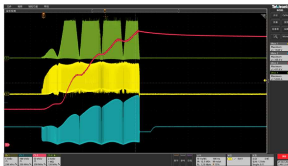
90VAC Input_0% Load_Startup CH1:VGS CH2:VDS CH3:VO-PFC CH4:IL-PFC
